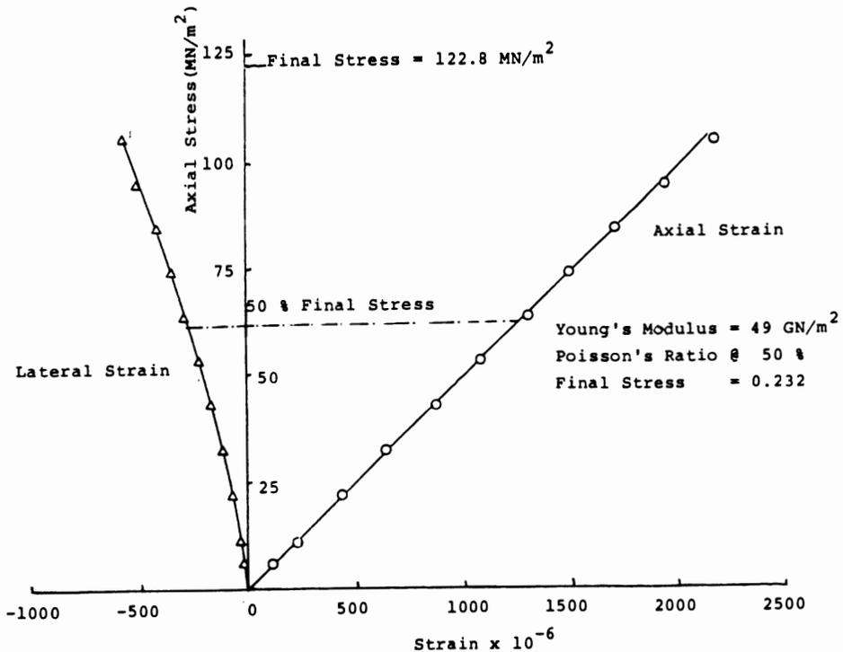
FIG. 1. Stress-strain relationship for specimen no. 2.
