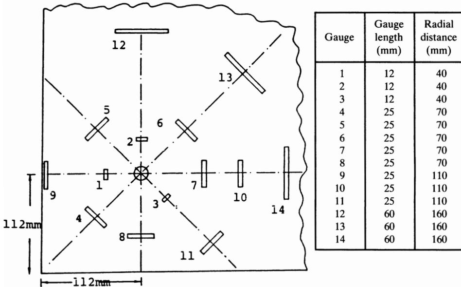
FIG. 2. Positioning of strain gauges around 14 mm dia. borehole.
